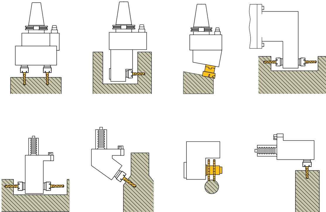
Special angle heads, multispindle heads, spindle speeders and driven tools custom developed according to workpiece drawings and machine specifications for drilling, tapping, light milling, heavy milling operations
