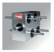
Globoidal cam mechanism with four synchronized output movements
