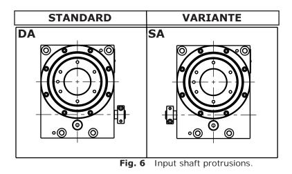
Unless otherwise stated, SERVO ROLLER POSITIONERS are supplied with the shaft extension at the DA position.
