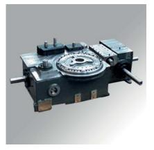
Mechanism with different types of cams that produce seven synchronized and intermittent synchronized movements at output
