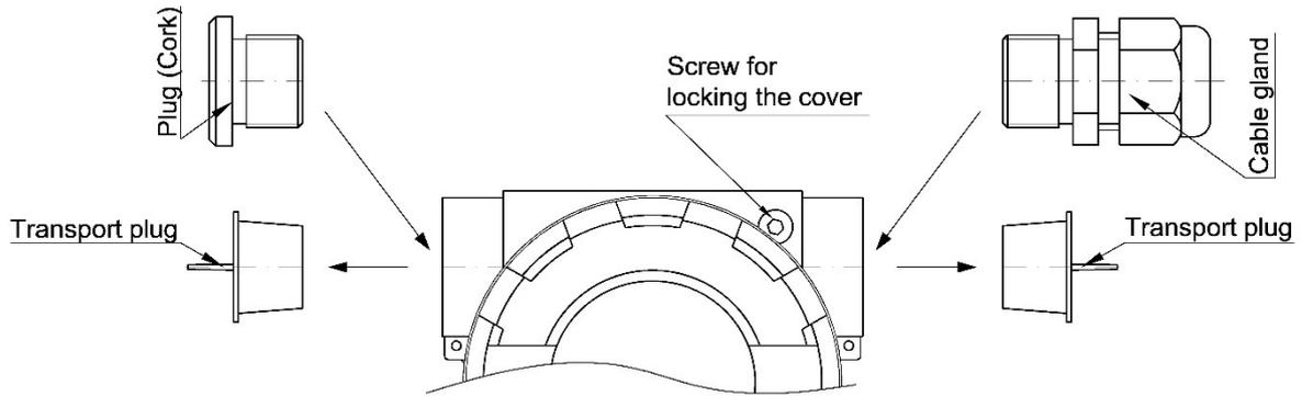
**Figure 7.** Installation of cable entries and blinding plugs
